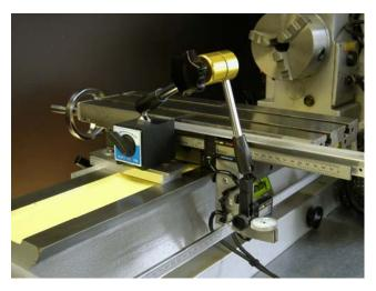
the horizontal plane of the lathe bed ways. Loosen the screws/bolts holding the encoder to its mounting and raise the "low" end slightly. (Don't let the shims fall out of position!) Repeat the above steps until the indicator readings are approximately the same. Tighten the encoder mounting securely. Now, take a break and admire your progress.
