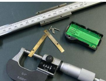
The other assembly will include the encoder circuit board, the battery, the buttons, and the encoder case or shell. This assembly, too, will hang together because the circuit board is held to the encoder case with screws.
