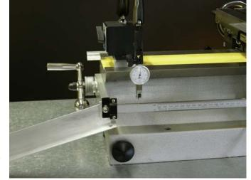
move the mounting in or out from the lathe bed (or add or remove shims under the mounting) until the indicator reading is the same when measured near the encoder and at the tailstock end of the beam. When the measurements are the same, tighten the fittings on the mounting securely.
